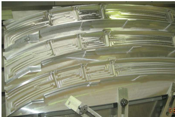
Fig. 19. Parts just after CNC machining
