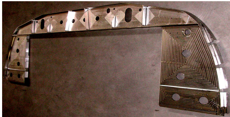
Fig. 8. The example of. Machining with \Phi 12mm cutter. Semi-finished product dimensions = 120mm x 752mm x 2400mm
