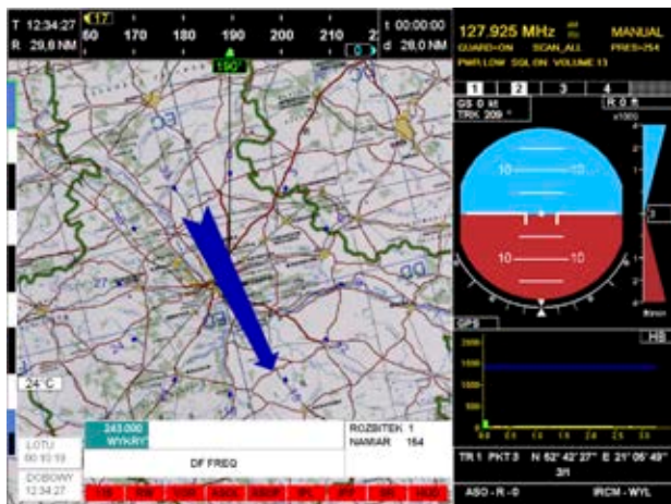
Figure 3. CSAR mode BEARING board showing relative bearing to the survivor (AFIT)
