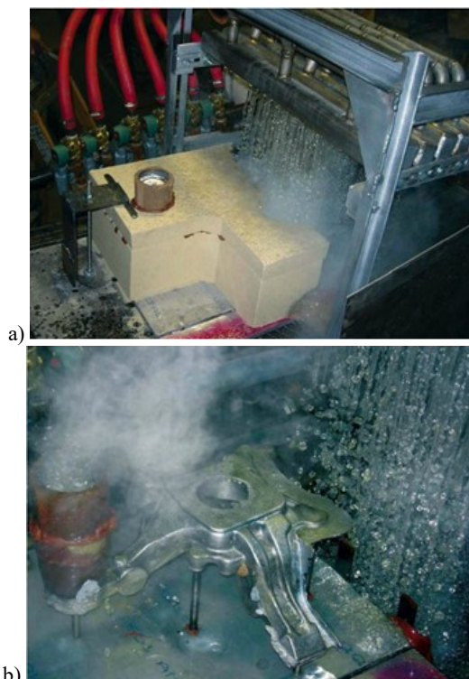
Fig. 1. The ablation casting process: a - the beginning of the ablation process, b - ready casting [8]
