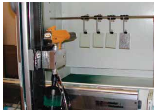
Fig. 6. Robotised electrostatic powder coating facility at CSIRO laboratories
