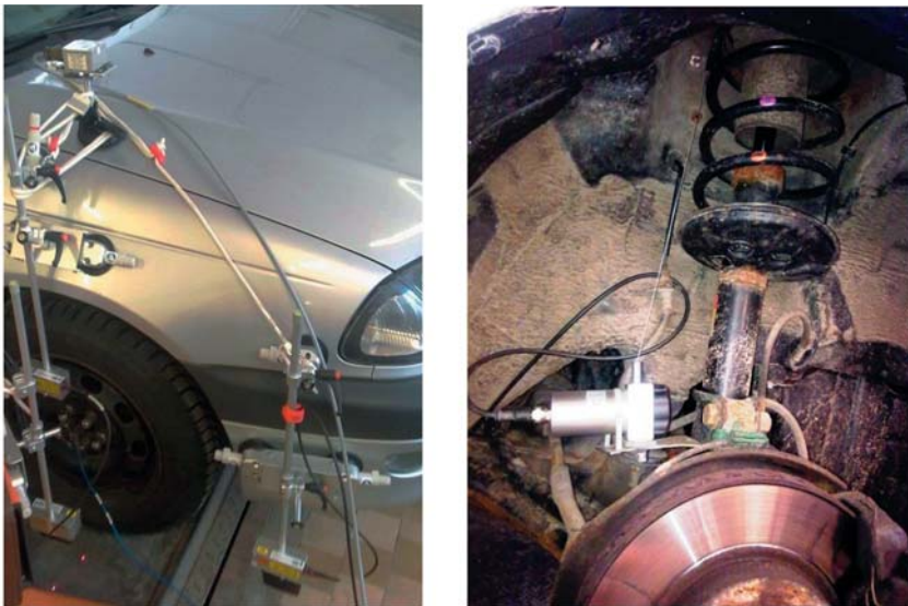
Fig. 2. On the left – on the test stand "Safeline 400/800" intended for measurement of shock-absorbers effectiveness. On the right – measurement of the car suspension travel
