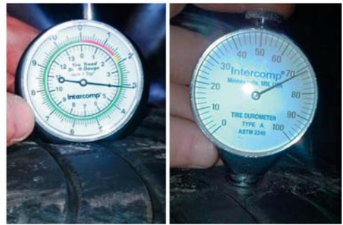
Fig. 4. Summer tyre tread depth and rubber hardness
