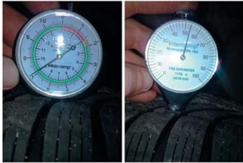
Fig. 3. Winter tyre tread depth and rubber hardness
