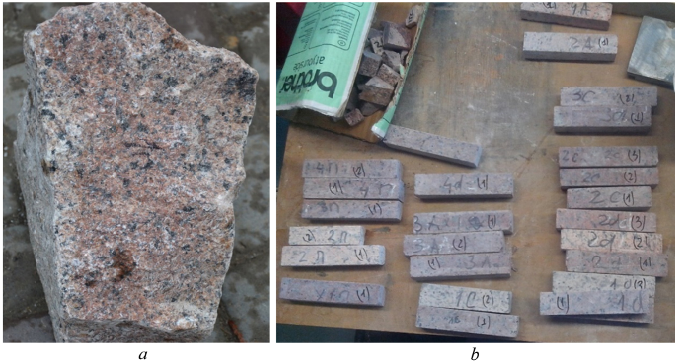
Fig. 3. Type of natural stone samples a – the kind of the sample selected at the quarry; b – the form of the stone bars made of the quarry samples
