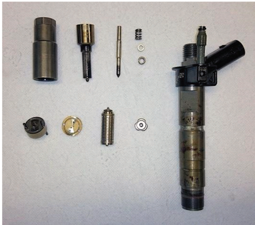
Fig. 2. Piezoelectric Bosch fuel injector disassemble on spare parts
