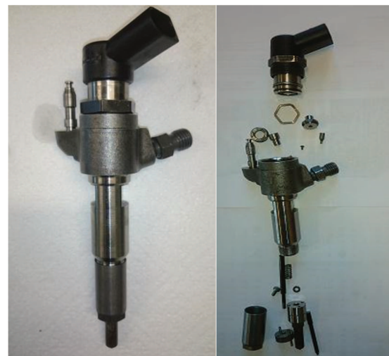
Fig. 5. A – Piezoelectric Continental VDO Siemens fuel injectors, B – Continental fuel injector disassembly on spare parts
