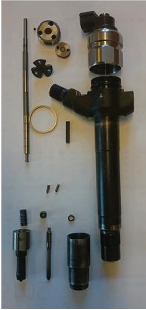
Fig. 7. Electromagnetic Denso fuel injector disassembly on spare parts
