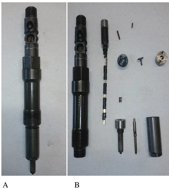
Fig. 8. A – electromagnetic Delphi fuel injectors, B – electromagnetic Delphi fuel injector disassembly on spare parts
