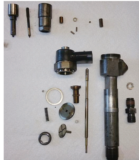
Fig. 4. Electromagnetic Bosch fuel injector gen. 2.1 disassemble on spare parts
