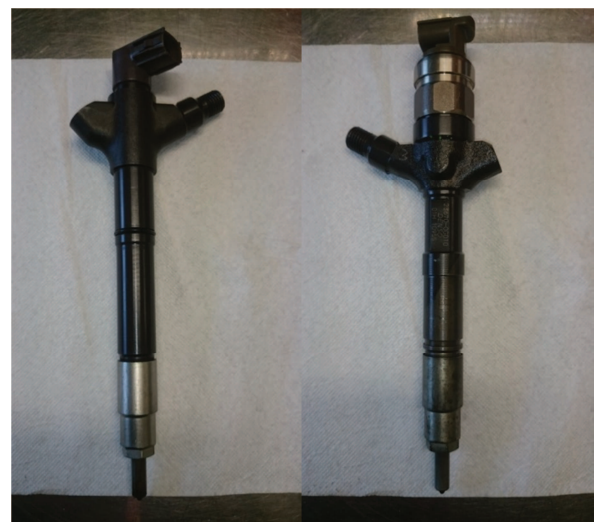
Fig. 6. Denso fuel injectors A – piezoelectric, B – electromagnetic
