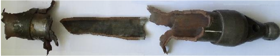
Fig. 1. The effect of a mortar projectile detonation inside a mortar barrel
