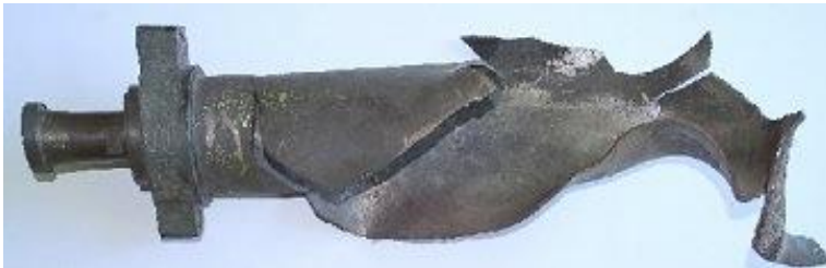
Fig. 14. Burst rocket motor of an LWD mine-clearing line charge
