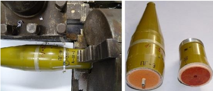
Fig. 10. Disassembly of a PG-9 projectile warhead by cutting; the same projectile warhead is shown cut open
