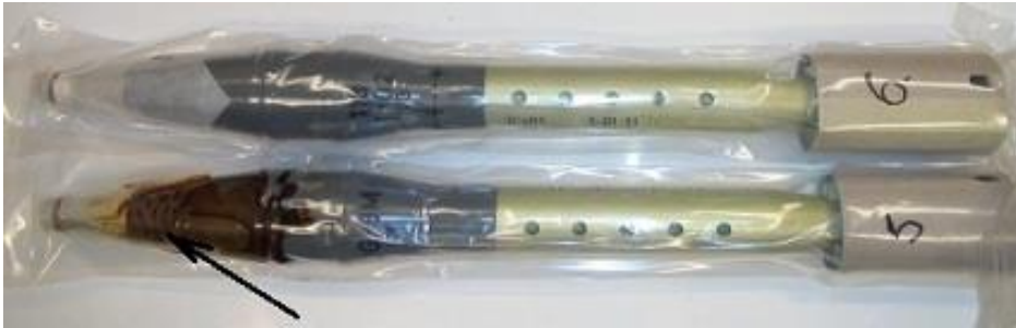
Fig. 4. TNT oil on the outer surface of an OG-9 projectile in a hermetically sealed plastic bag
