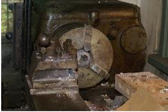
Fig. 11. A part of the GROM SAM warhead remaining in a lathe chuck
