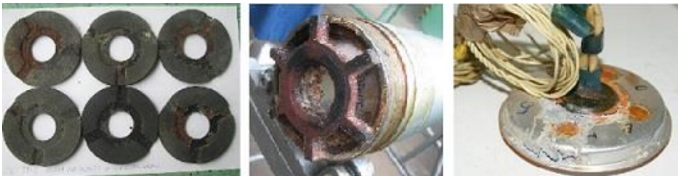
Fig. 3. Defective plastic pad and the effects of its installation in the rocket motor of an M21 missile
