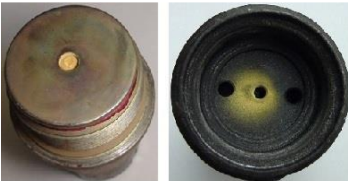
Fig. 12. High explosive dust inside the fire hole of fuze head (a) and around the fire hole (b) in the body of an RGM fuze
