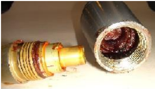
Fig. 5. TNT oil on the thread form of an OG-9 projectile
