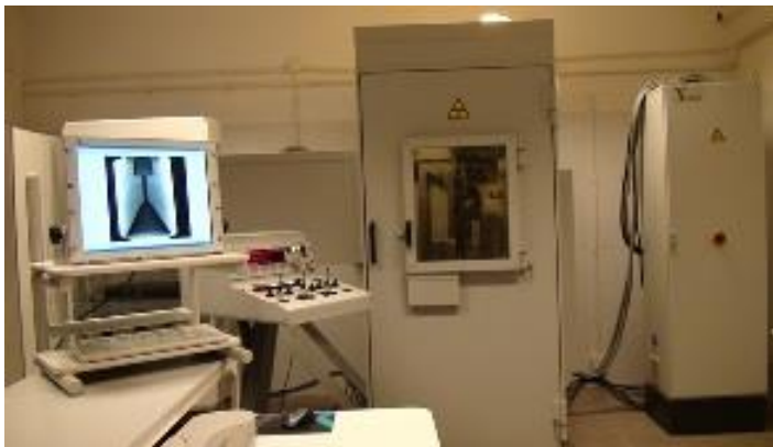
Fig. 6. Munition radiographic examination workstation
