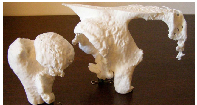
Fig. 7. Pelvic bones model made by MEM technique
