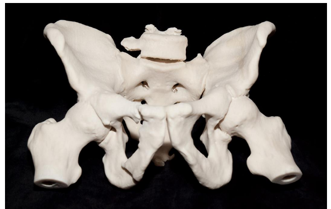
Fig. 6. Pelvic bones model made by 3DP technique – wall-thickness 4 mm
