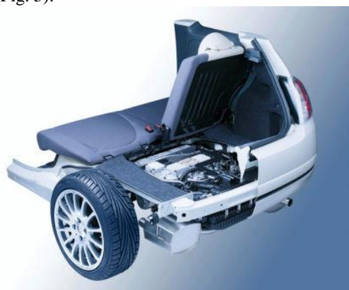
Fig. 5. Cross-section of rear end of Fiat 500 with KSPG - FEV Range Extender [12]
