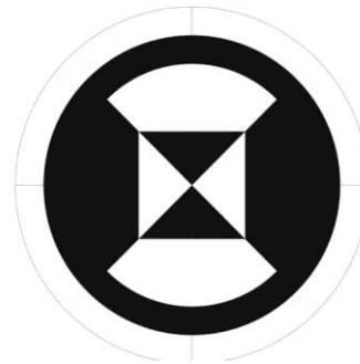
Fig. 9. Using Autonomous vehicles can independently determine their exact location with the so-called landmark signs
