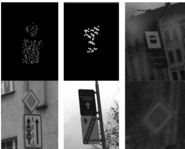
Fig. 8. Using LIDAR detection for different traffic signs (Landaa and Prochazkaa, 2014)
