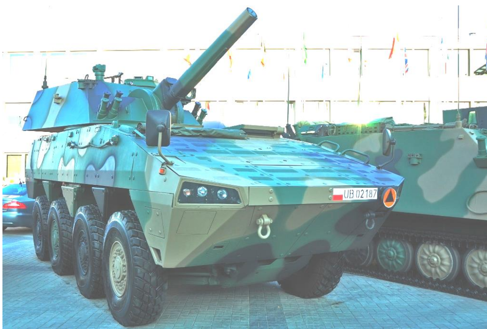
Fig. 1. 120 mm self-propelled mortar Rak on KTO Rosomak undercarriage (fot. HSW-CPW)
