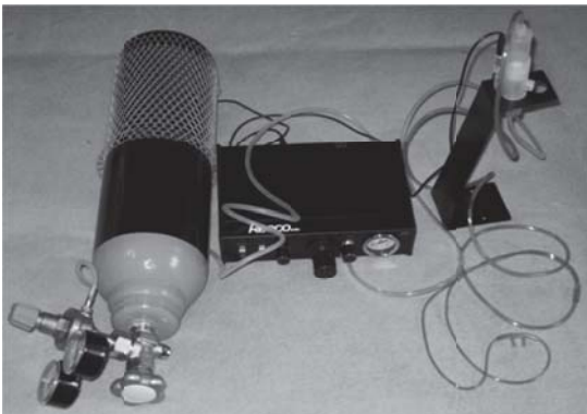
Fig. 3. Prototype of odour sample dispenser.
