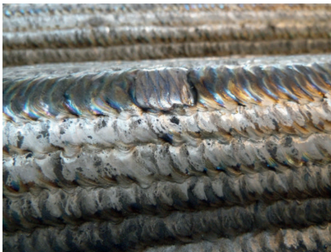
Fig. 2. Piping in the surfacing weld repaired manually by the 141 method Source: own collections
