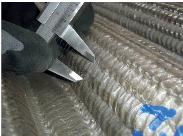
Fig. 6. Measurement of the beads' thickness Source: own collections
