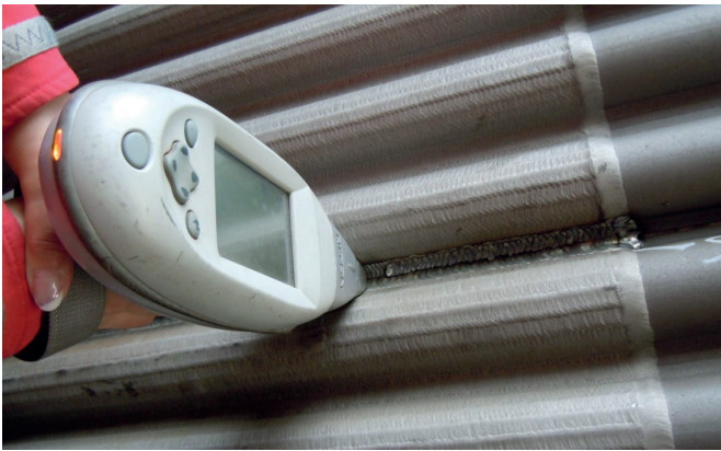
Fig. 13. Examining an iron content on the surface of the surfacing weld by the X-ray spectrometer
