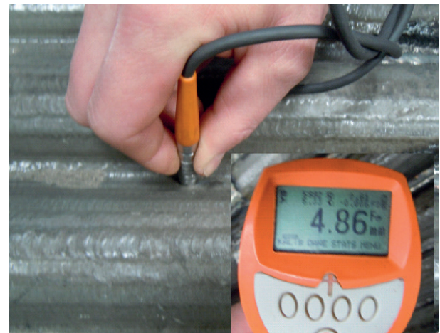
Fig. 11. Measurement of the thickness of the Inconel 625 surfacing weld on the flat bar
