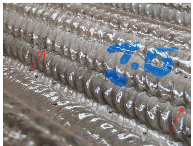
Fig. 8. Systematic irregularities on the beads' boundaries – "fastener effect" Source: own collections
