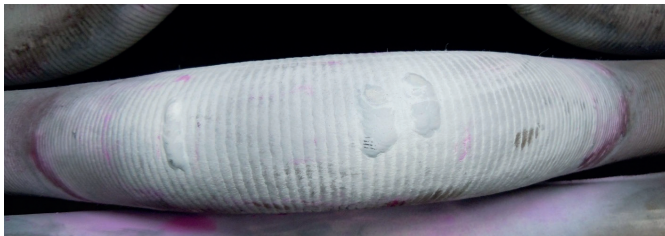
Fig. 17. Cracks after bending repaired by the 141 method
