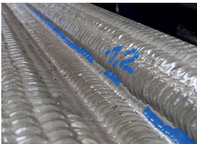
Fig. 10. An area on the beads' boundaries of an insufficient thickness Source: own collections
