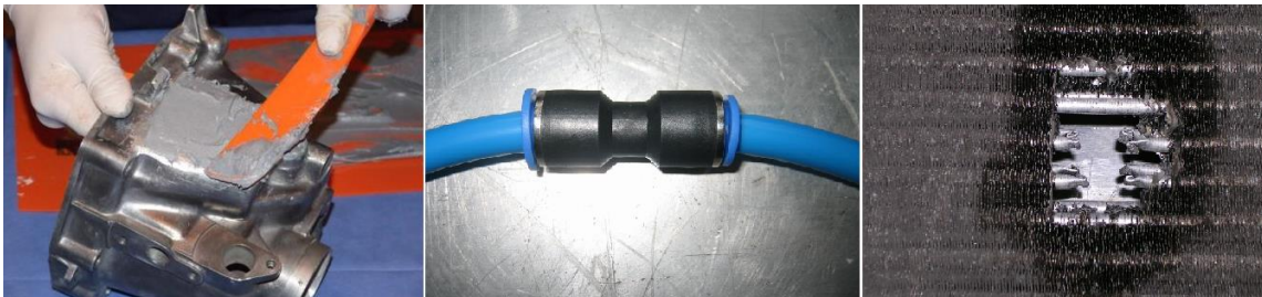
Fig. 3. Sample methods of expedient repairs: hulls with adhesive composites (left), lines with fast-joints (middle) and radiators with bent or damaged lines
