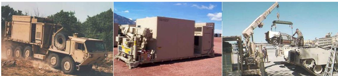
Fig. 4. FRS on a HEMTT-type vehicle during transportation (left), working post after removal from the transporting vehicle (middle) and during repair works (right)
