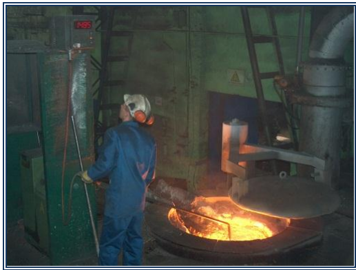
Fig. 4. Furnace. Temperature checking
