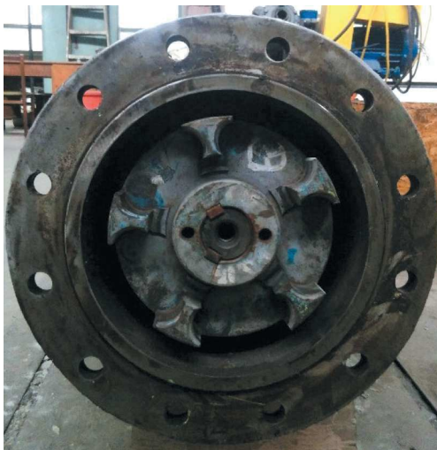
Fig. 2. View of passive member of insert clutch used in roadheader
