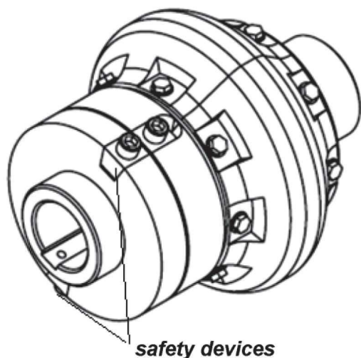
Fig. 12. Raptor-SK clutch with fuses [8]
