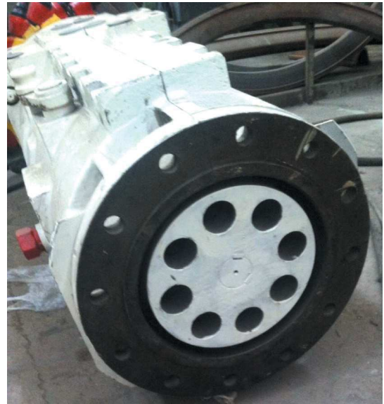
Fig. 3. View of passive member of finger clutch used in roadheader
