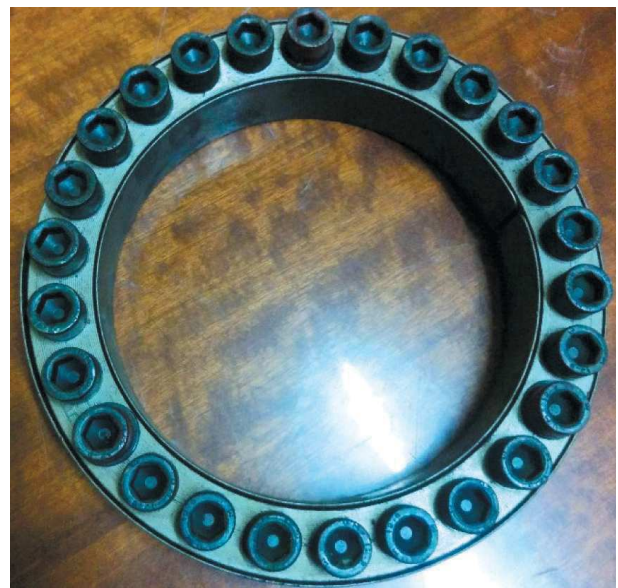
Fig. 4. View of expansion ring for use in head of mining roadheader
