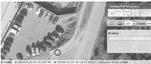
Fig. 3. GCP and ICP collected using Polish Geoport of Spatial Data Infrastructure
