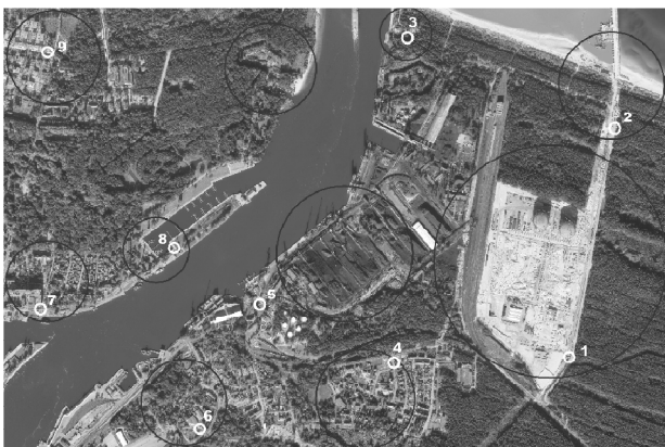
Fig. 2. Ground Control Points (GCP) collected across field surveying
