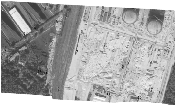
Fig. 6. ICP used to assess of accuracy of orthophotomap
