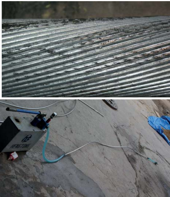
Fig. 13 Broken-out section view of umbilical after test
