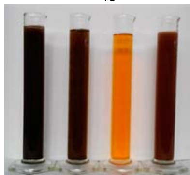
Fig. 4. Tar waters from the biomass gasification installation
