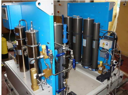
Fig.1-2 Configuration of the breathing air supply and treatment equipment of the DGKN – 120 complex. Source: own study.
