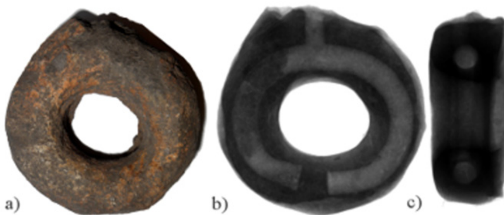
Fig. 5. Casting mold with damaged gating system (a); X-ray image of mold cavity – front view (b) and side view (c) [6]
