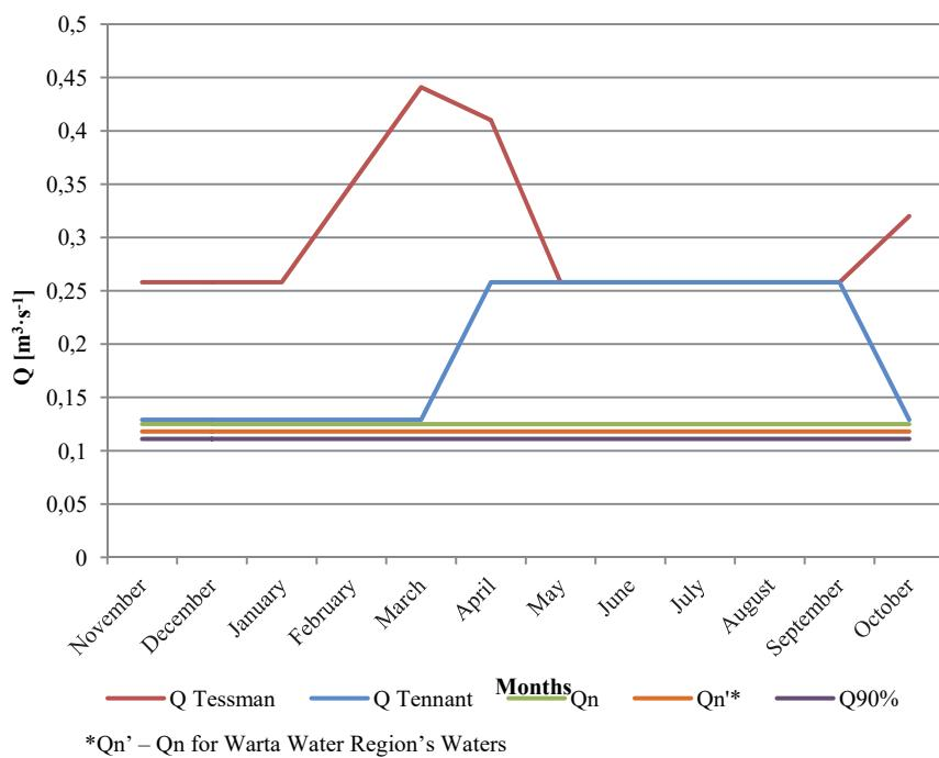
**Fig. 5.** Environmental and instream flow rates in Mała Wełna river at Kiszkowo cross-section
