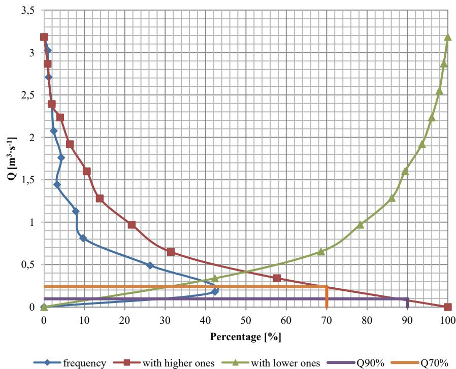
**Fig. 4.** Flow duration curves for Mała Wełna river at Kiszkowo cross-section in 2000-2010 period
