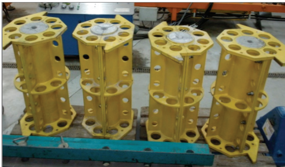
Fig. 8. Split bushings filled with concrete
