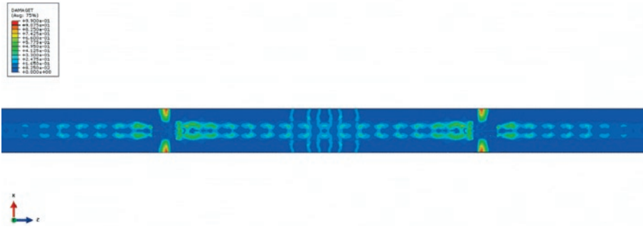
Fig. 15. The final picture of the material damage caused by the maximum external load (top view of the slab): stiffness degradation section
