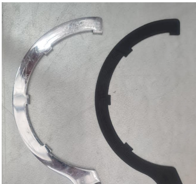
Figure 11. An example of reproduce of specialist tool using 3D printing Source: Authors' own work.
