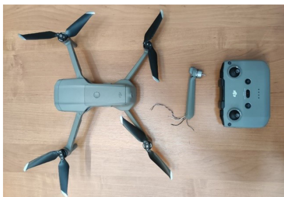
Figure 7. Unmanned aerial vehicle and damaged arm for repair Source: Authors' own work.
