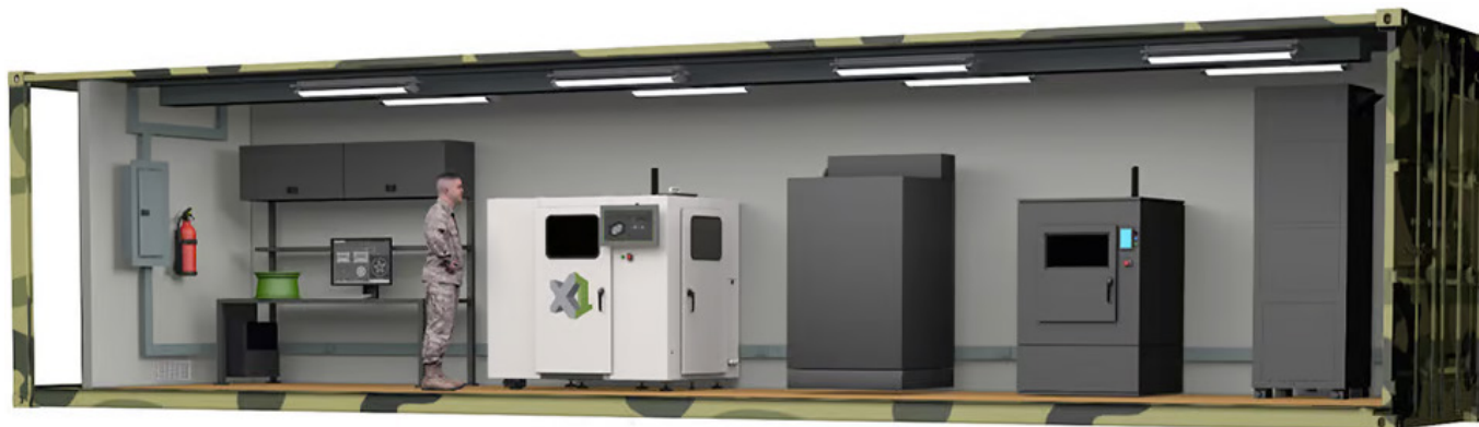
Figure 10. Container, mobile additive printing house designed by ExOne for the United States Department of Defense. Adopted from: “Wojskowe zastosowanie druku 3D” by M. Maciążek. Copyright 2021 by Publisher. https://3d.edu.pl/wojskowe-zastosowania-druku-3d/
