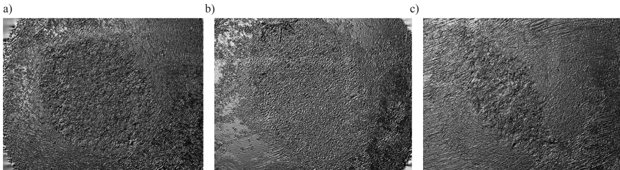
Fig. 11. Images of the wear traces on the \text{Al}_2\text{O}_3 ball for TDF: a) Ti, b) Ti6Al7Nb, and c) Ti13Nb13Zr
