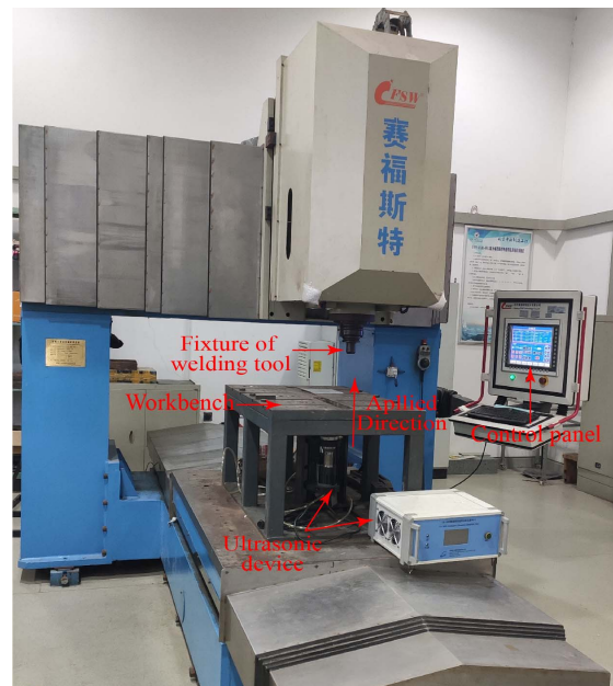
Fig. 1. FSW equipment with ultrasonic device
