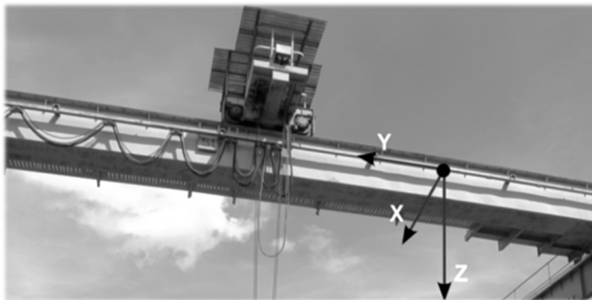
Fig. 8. Axis of measurement system for test object (Experimental research crane – OBRDiUT "Detrans" in Bytom)
