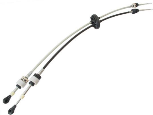
Fig. 1. Gear shift cable - research company product (company internal material)
