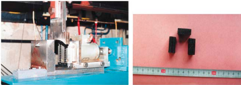
Fig.4. Preparation for shear stress tests and brake pads samples ready for investigation of mechanical characteristics
