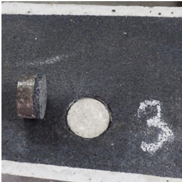
Fig. 11. Failure between the geotextile anchor layer and the elastomer material of the pad (failure type B/C)
