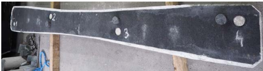
Fig. 6. Prestressed concrete sleeper PS-94 with attached prototype SBR-based USP (variant II) after the pull-off test, with marked location of four measurement points
