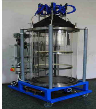
Fig. 1. The BKB 100 bioreactor used in the research
