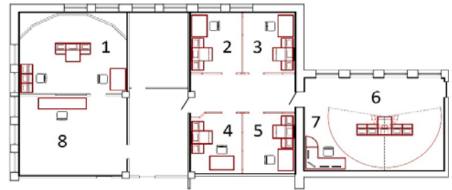
Figure 5. Navigation simulator lay out: (1) bridge No. 1, (2-5) bridges No. 2 to No. 5, (6) bridge No. 6, (7) instructor workplace, (8) instructor workplace and debriefing room.
