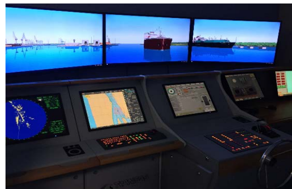
Figure 8. Bridges from No. 2 to No. 5 with 3-channels 120° horizon visualisation
