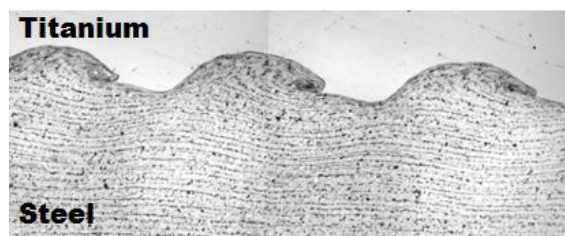
Fig. 1. Example of interference zone of explosively clad steel-titanium
