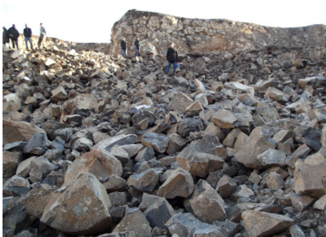
Fig. 4. Rock pile of blast round with drill cuttings stemming at Asagi Caglayan basalt quarry
