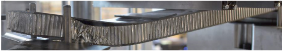
Fig. 3. Flexure failure mode (a) and core shear (b)
