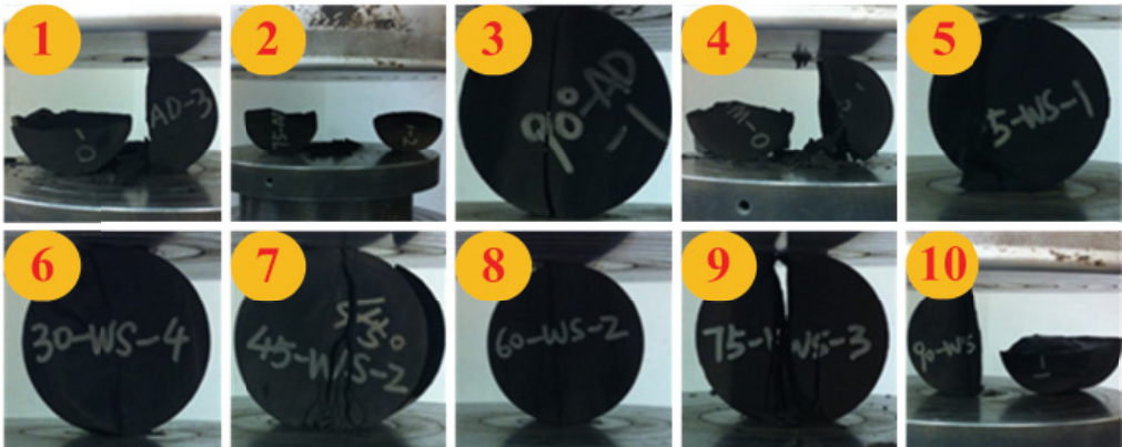
Fig. 9. Failure types in the Brazilian test Self-Elaboration
