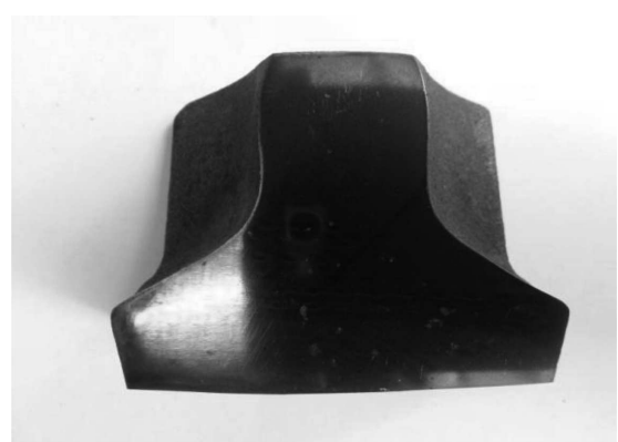
Fig. 3. Cross-section of a single tooth in the gear assembly
