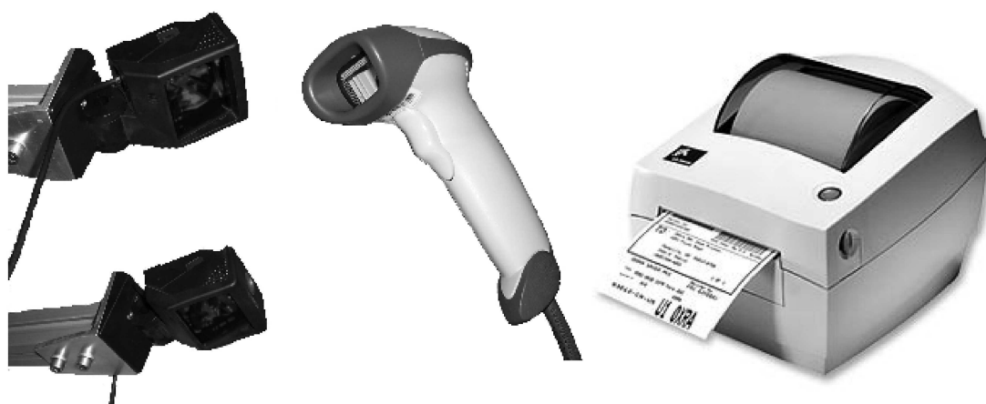
Fig. 7. Barcode subsystem – scanners and Zebra barcode label printer
