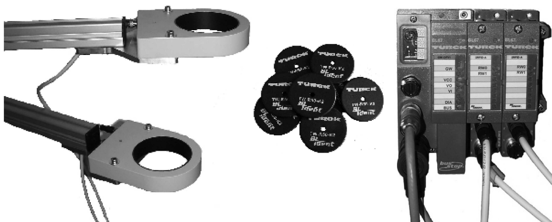
Fig. 6. RFID subsystem – antennas, passive tags and RFID controller
