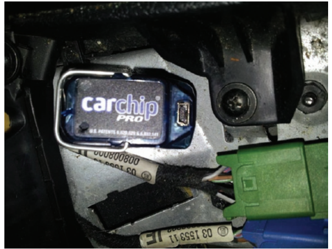
Fig. 3. CarChip Pro Recorder in a vehicle's OBD slot
