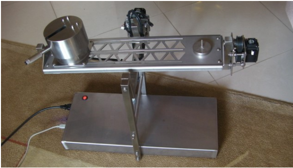
Fig. 5. Physical model of the ship gun – implementation
