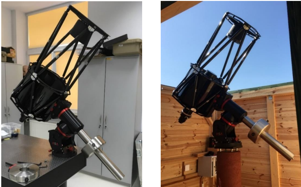
Fig. 2. NFOV telescope on a laboratory and field test stand
