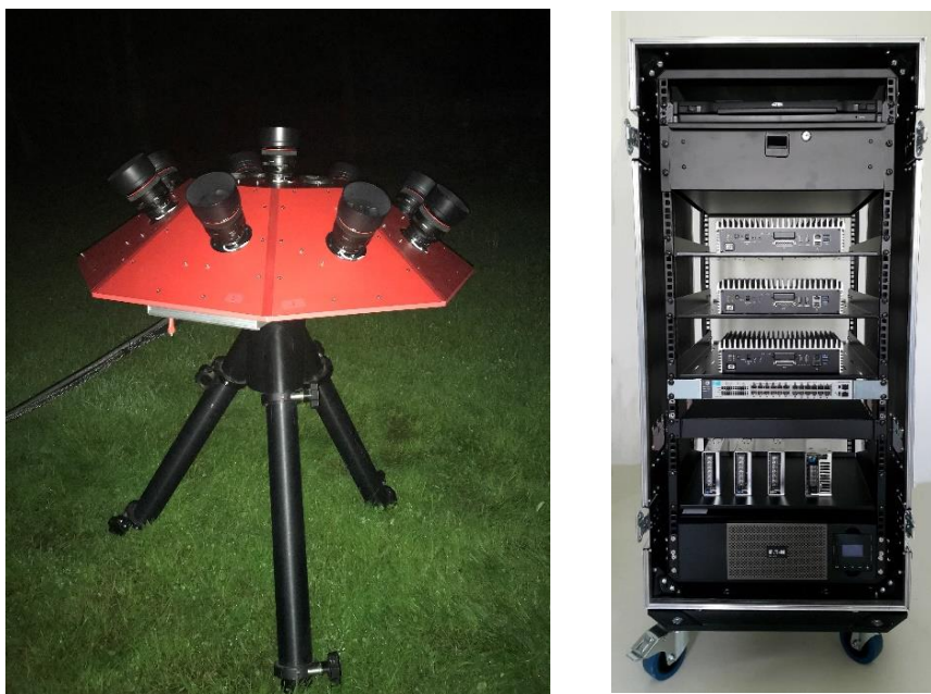
Fig. 1. Mechanical assembly for the WFOV - next to a rack with a system of control computers and a time server
