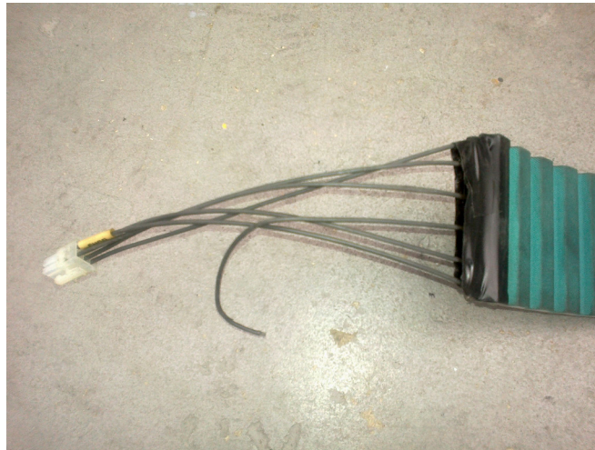
Fig. 2. Timing belts in robotics, with signal cable in cord layer [15]
