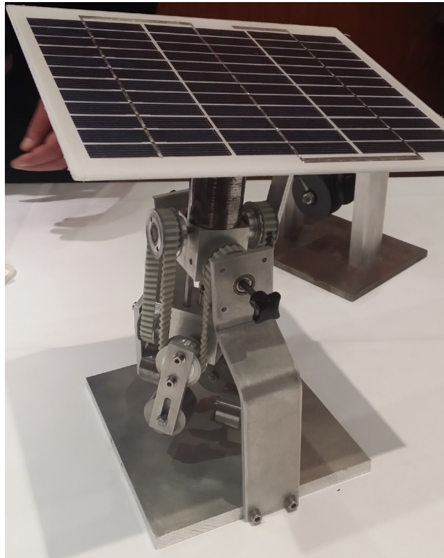
Fig. 1. Solar panel regulation system
