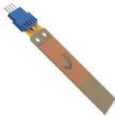
Fig. 8. V21BL-ND piezoelectric converter (dimensions in inches) [6]
