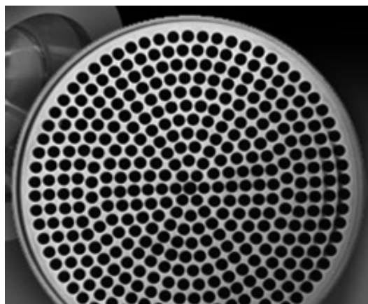
Figure 1. Typical breaker plate holes (Source: JoeTools, 2009)
