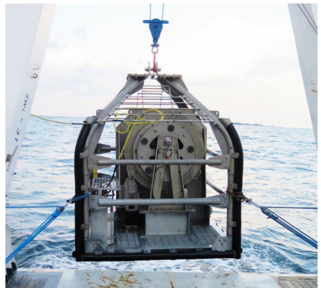
Fig. 2b. The NEPTUNE 5000 penetrometer by the R/V IMOR ship's side
