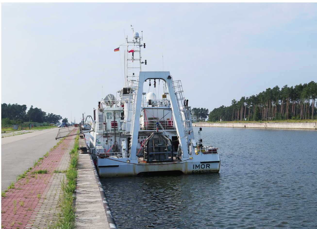
Fig. 5. The RV IMOR vessel with an A - frame visible on its back
