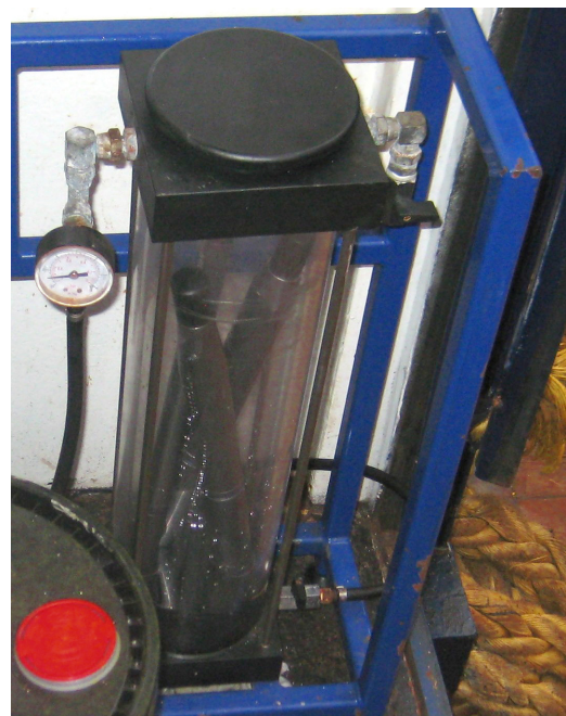
Fig. 3. Measuring tips inside a vacuum chamber
