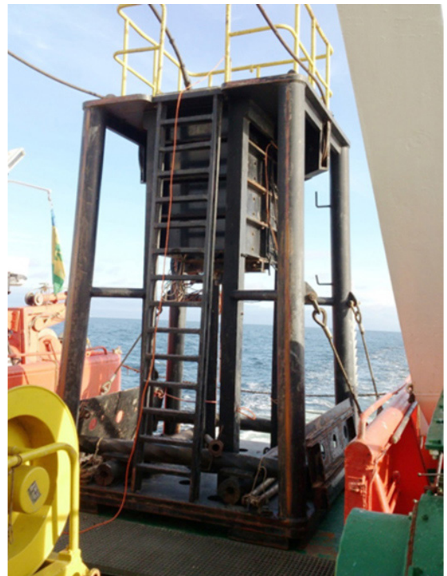
Fig. 1. CPTU ROSON penetrometer by the A.P. Van den Berg company situated on board of the R/V St. Barbara survey vessel.
