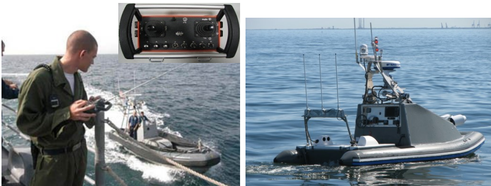
Fig. 3. The manual control of the USV 'Edredon' from a ship's deck [R&D project No. 0 R00 0004 07 documentation]
