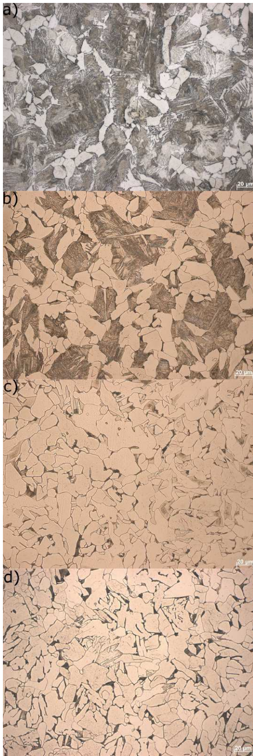
Fig. 3. Microstructure of the steel after isothermal holding for the shortest time at temperatures: a) 800°C, b) 750°C, c) 700°C, d) 650°C
