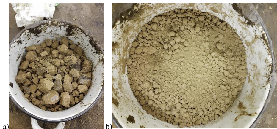
Fig. 2. Batch preparation: a) contaminated bleaching earth before crushing process b) contaminated bleaching earth after the crushing process
