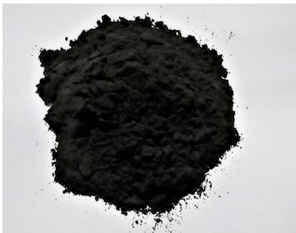
Fig. 8. Purified bleaching earth after the pyrolysis process
