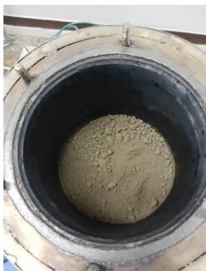
Fig. 3. Bleaching earth after low-temperature pyrolysis
