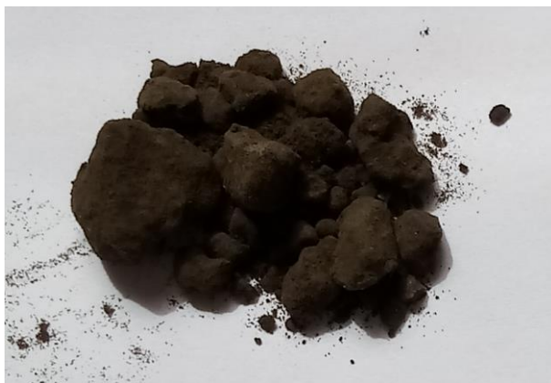
Fig. 7. Bleaching earth after the paraffin refining process
